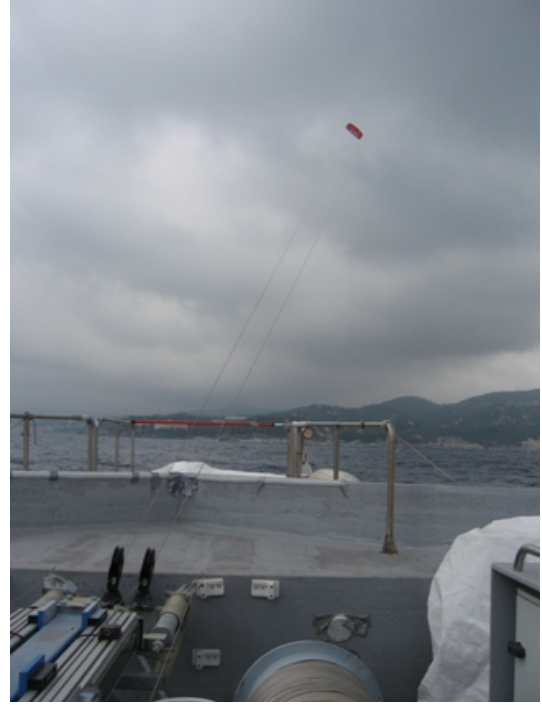
Figure 8: KE-yoyo small scale prototype operating in Liguria, Italy, mounted on a boat.
