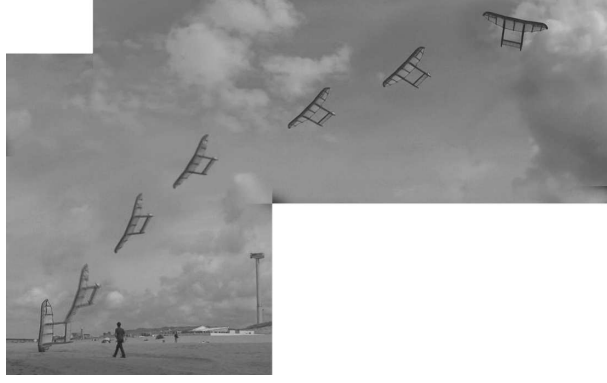
Fig. 17: Composite photo constructed from flight test footage with v_W \approx 6 \text{ ms}^{-1} , the flight time captured in this figure is approximately 12 s.
