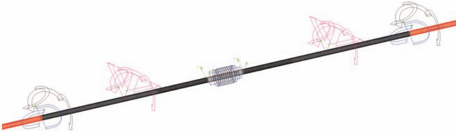
Figure 4.4: The complete cable model incorporating elasticity.
